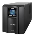
APC Smart-UPS C, Line Interactive, 1000VA, Tower, 230V, 8x IEC C13 outlets, USB and Serial communication, AVR, Graphic LCD
